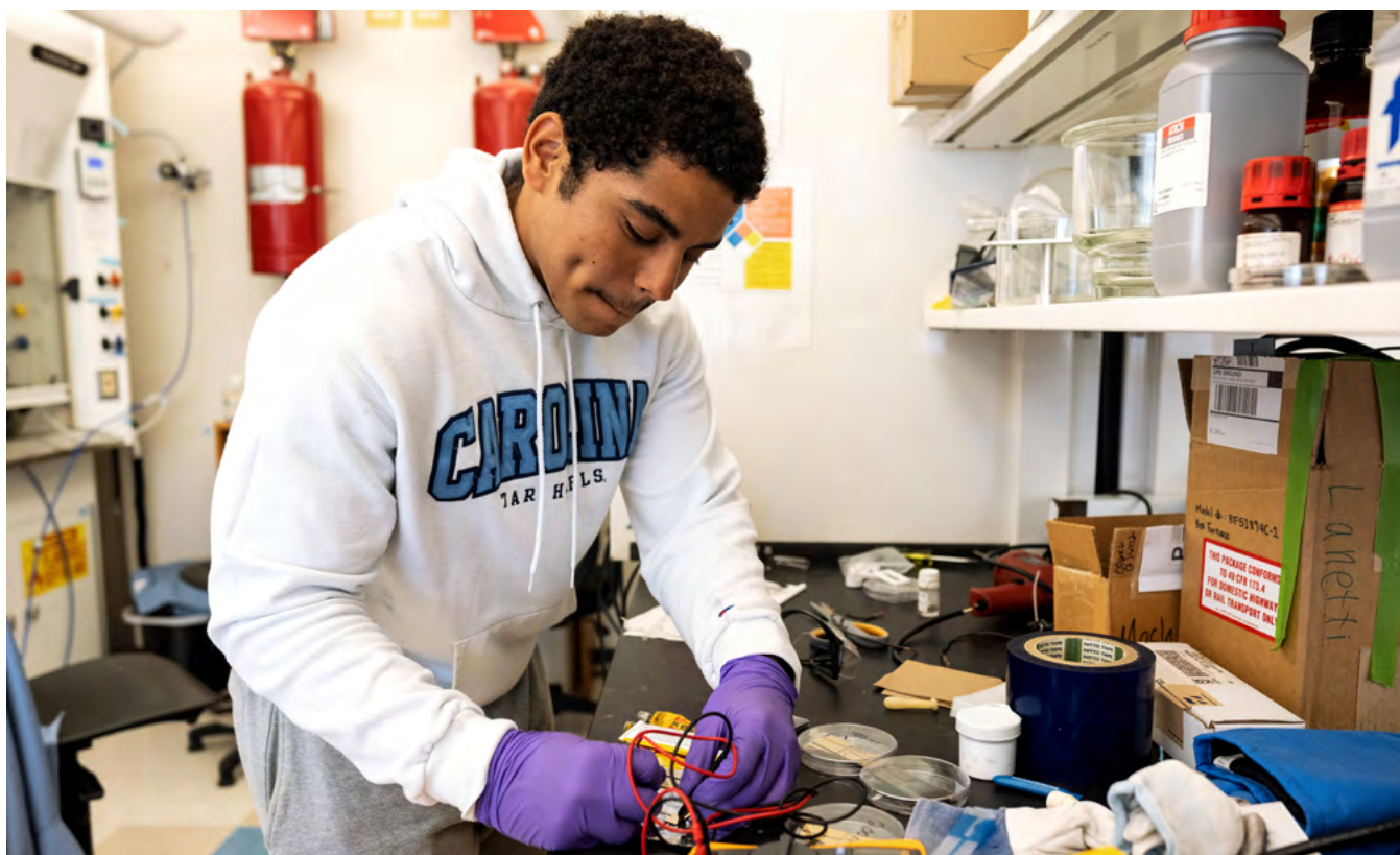
Miguel Reyna, a junior chemistry major from Fayetteville, North Carolina, works in the Scott Warren Lab in Kenan Labs. July 5, 2023. Reyna is researching intercalation in batteries he builds using titanium, Teflon, graphite and liquid lithium on a glass laboratory slide.
