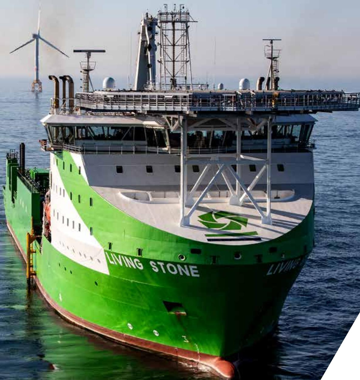
The multifunctional cable-laying vessel Living Stone is the first in the industry to run on LNG.
