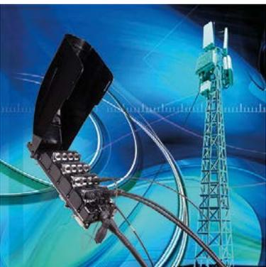
The MASTERLINE Ultimate Hybrid High Voltage (MLUH HV) hybrid cable system has been designed specifically to meet the significantly higher power requirements of 5G mobile cells. This hybrid cable transmits data using fiber optics and supplies the remote radio heads (RRH) with 230 V AC voltage instead of the 'traditional' 48 V DC voltage. This significantly reduces power loss of the cable and thus the carbon footprint of the telecommunications providers.
