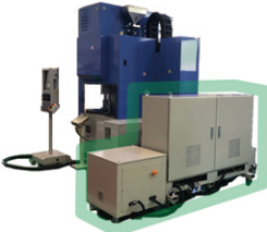
Dedicated molding machine power stabilizer
