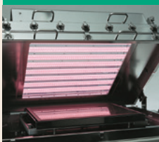
Panel photo-cleaning equipment
