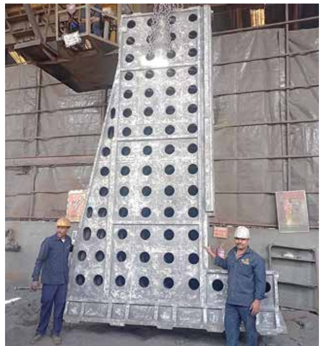
Higher weight single piece castings (up to 14.28 MT) from WIL Foundry
