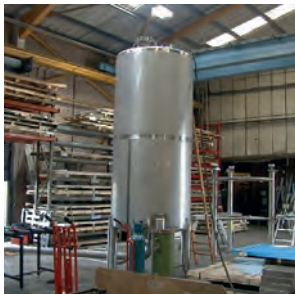
Stainless steel storage tank
