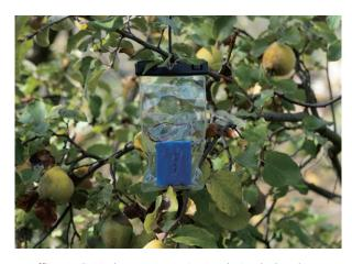
An offline AudioMoth acoustic monitoring device deployed on a fruit tree on a farm in Italy
